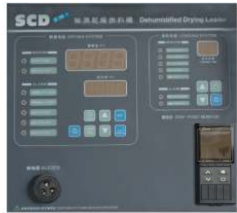
Optional panel with dew-point monitor
