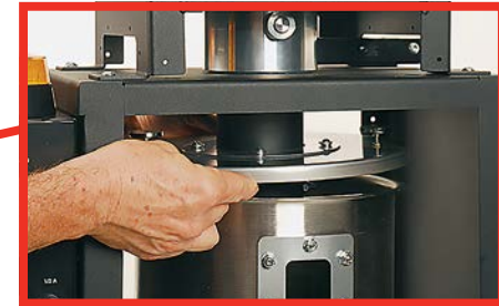
Magnetic retainers on hopper enclosure allow rapid access to LIW Hopper.
